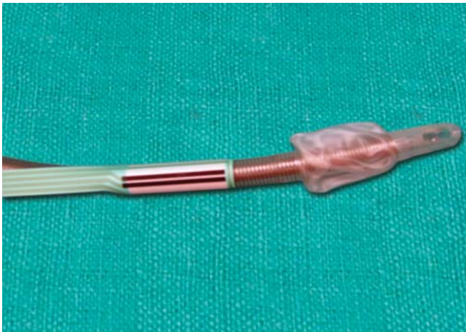
Fig. 3: Amplified image of the endotracheal tube with two integrated stainless steel contact electrodes on either side of the tube located above the endotracheal tubes cuff
